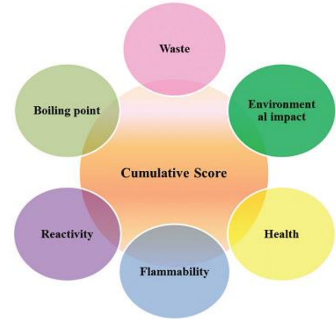
Fig. 2 Various properties employed to calculated the cumulative score of each solvent listed in GSK's SSG.
